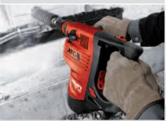
Plenty of power for drilling through-holes efficiently with breach bits up to 80 mm dia.
